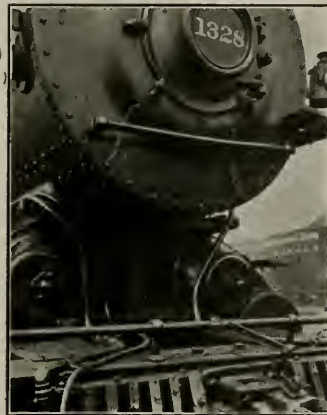
CAST IRON FRONT END OF LOCOMOTIVE SHOWING CRACKS WELDED WITH U. S. L. ARC WELDER WITHOUT REMOVING FROM LOCOMOTIVE.
